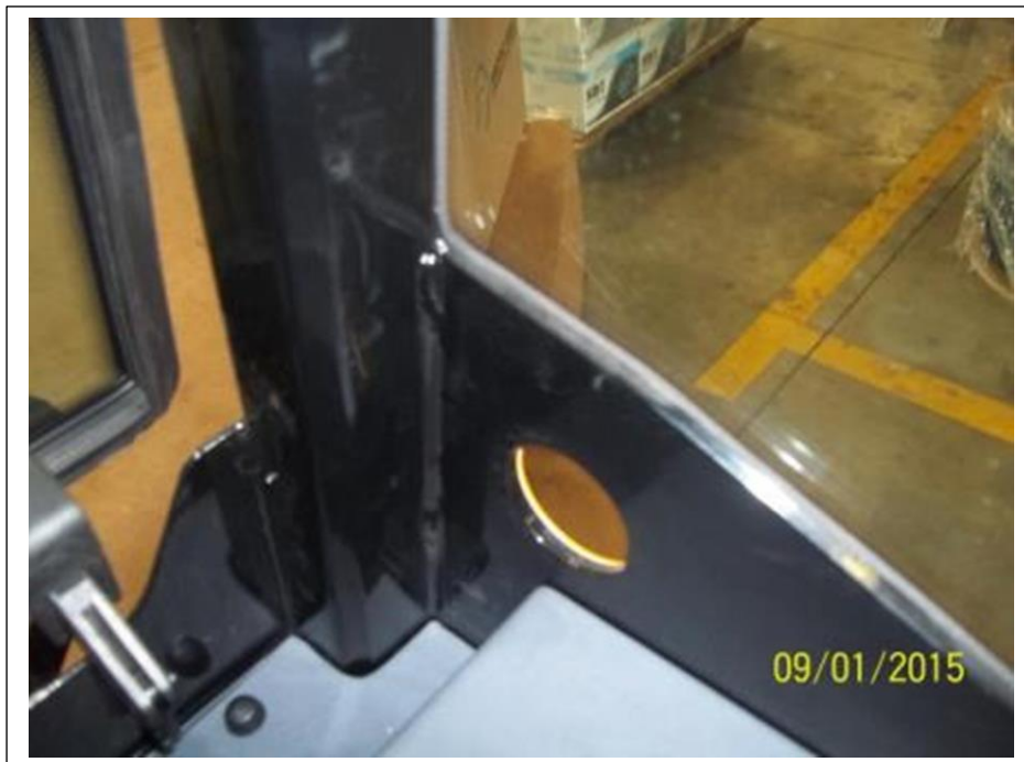
Door stop removed
