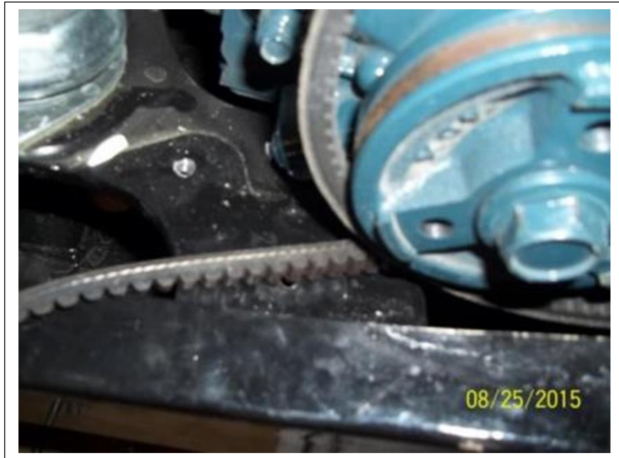
Insert the belt prior to installing the compressor drive pulley.
