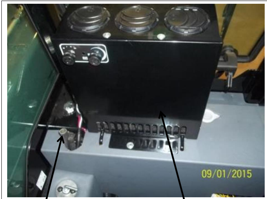
Hoses and wiring for evaporator.
